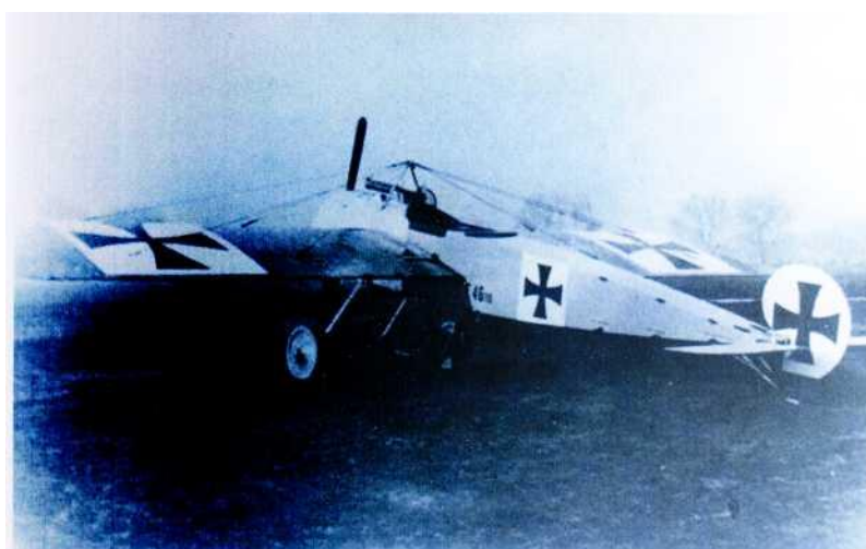
The longer "bathtub" cockpit of the M.5K/MG (E.1) is quite evident. This aircraft was serialied 46/15.
